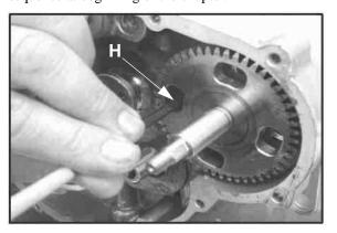
NOTE: Occasionally spin the oil pump when installing bolts to check for binding of the rotors.
